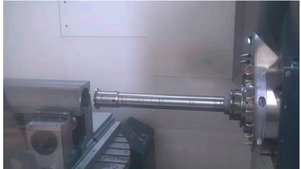
Finishing (before honing)
